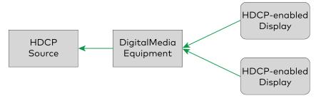
Devices that retransmit HDCP content must inform the source of all the downstream connections in the system. Every HDCP device has a unique ID, know as a Key Selection Vector (KSV), that must be passed to the source. The source must then verify each device before it transmits content. It is this authentication process that causes the switch time delay in HDMI devices.
