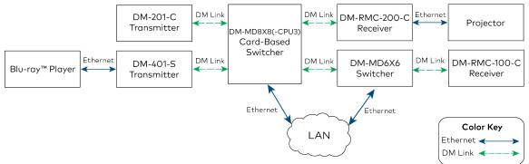
The main Ethernet uplink to a DM system occurs at the DigitalMedia switcher.
