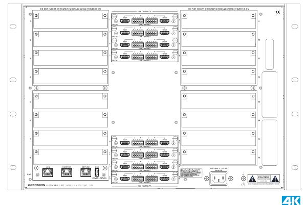
\* Crestron offers a new set of DM 4KZ cards and endpoints that enable new and existing DM systems to handle full 4K60 4:4:4 video signals, as well as HDR video signals (HDR10), without having to replace any wiring or switchers. The term "4KZ" refers to 4K60 4:4:4 and HDR video signal support.
