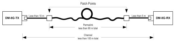
**NOTE:** Total patching should not exceed 33 ft (10 m). Patching on the DM 8G RX side should not exceed 16 ft (5 m).
