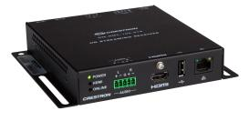
The DM-RMC-100-STR is a compact H.264 streaming decoder designed to receive high-definition AV signals over an IP network. It is a perfect complement to any DigitalMedia switcher with streaming output and can also be used to add streaming input capability to other switchers and devices.
