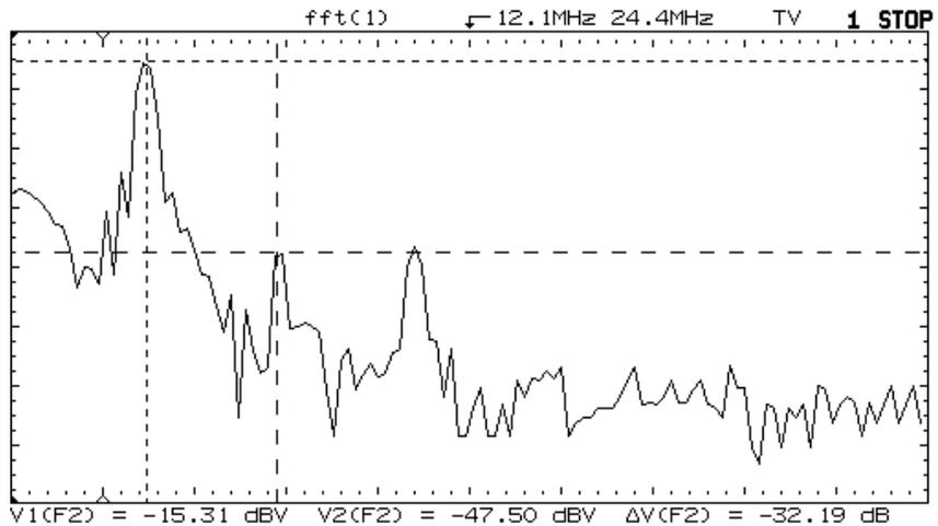
**The FFT function shows that the harmonic content of the color burst is more than 31 dB below the subcarrier**
