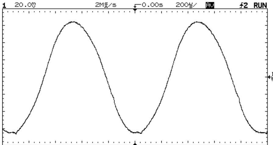
**On this waveform, 256 averages were used to reduce the noise**
