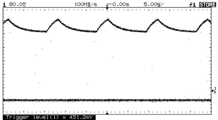
This is a triggered view of the asynchronous noise shown in figure 2-17.
