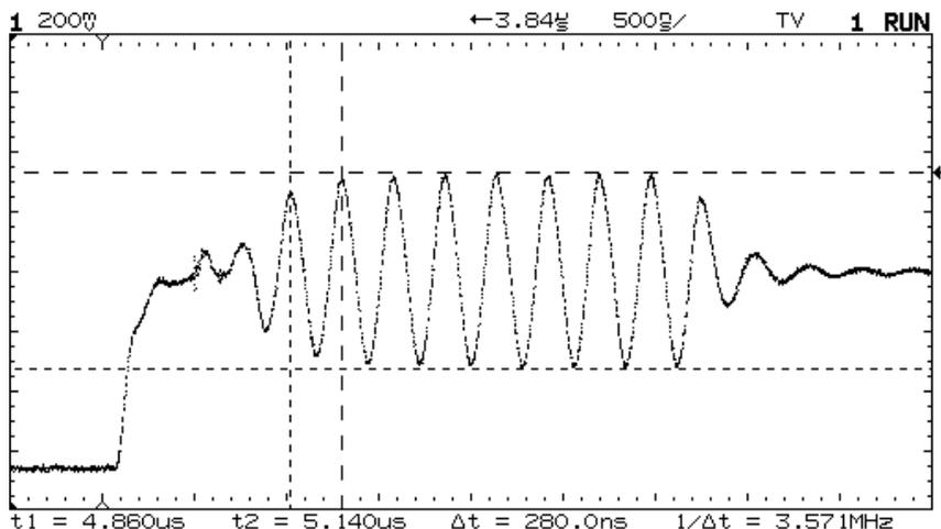
The scope controls are used to zoom in on the color burst in the time domain
