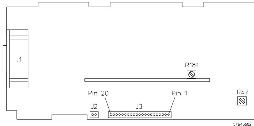
**Low Voltage Power Supply connector J3 pinout**
