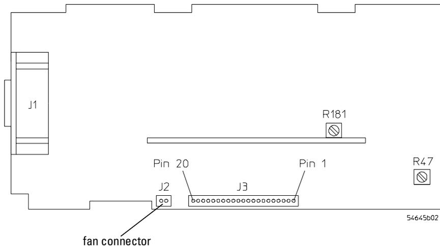
**Low Voltage Power Supply fan connector location**
