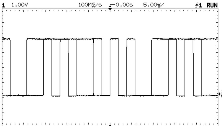
Stable trigger, but the waveform is not synchronized with the trigger
