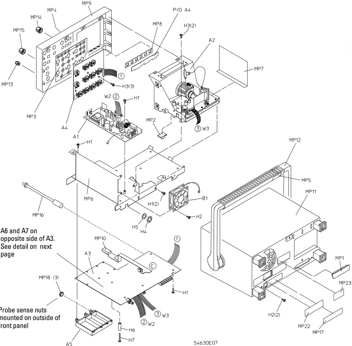
Exploded view of oscilloscope
