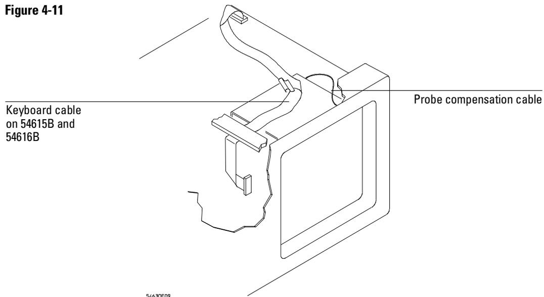
**Positioning keyboard cable on 54615B and 54616B**
